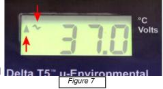
a [~] will appear on the numeric display (Figure 7). Pressing the down arrow will toggle the disable of the power interrupt. When the power interrupt is disabled a [^] will appear on the numeric display (Figure 7) but the control current will continue. Note: The Reset LED will flash if the controller goes into alarm. This feature cannot be disabled.
