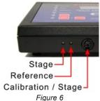
plug on the front of the controller (*Figure 6*) will adjust the Reference circuit. When calibration is complete you can remove the calibration plug and re-insert the stage adapter plug.
