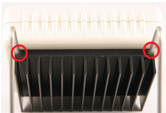
Locations to install controller stand
